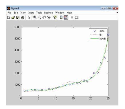
Since the data is closely correlated but not exactly linearly dependent, the fit curve (dashed line) shows a close, but not an exact, fit. The fifth-degree polynomial curve, newfit, is a more accurate mathematical model for the data.
